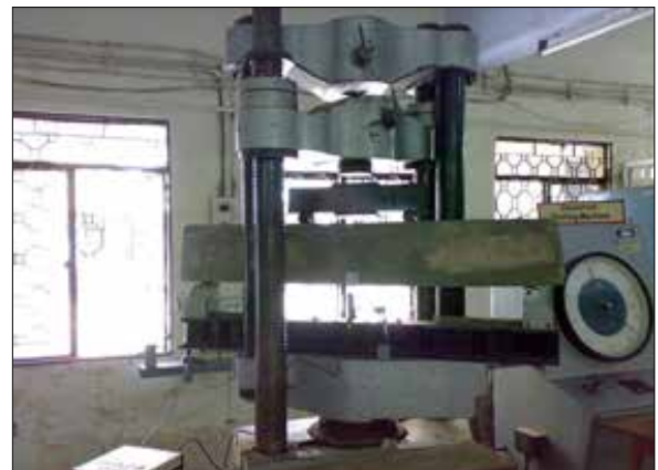
Figure 2. Loading arrangement for testing beam
