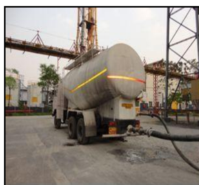
Fig 7 : Fly Ash Bulker Unloading
